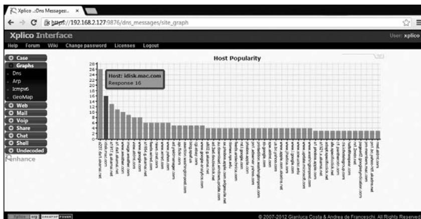
Figure 7-23: Xplico graphs DNS queries by frequency.
