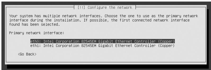
Figure 4-15: Selecting the primary network interface
