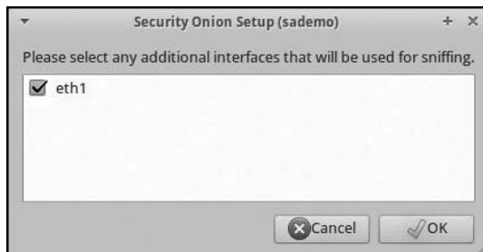
Figure 3-14: Selecting the sniffing interfaces
