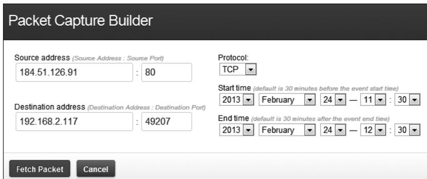
Figure 8-16: Packet Capture Builder window in Snorby
