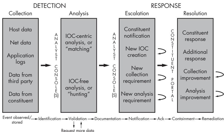
Figure 9-2: NSM process
