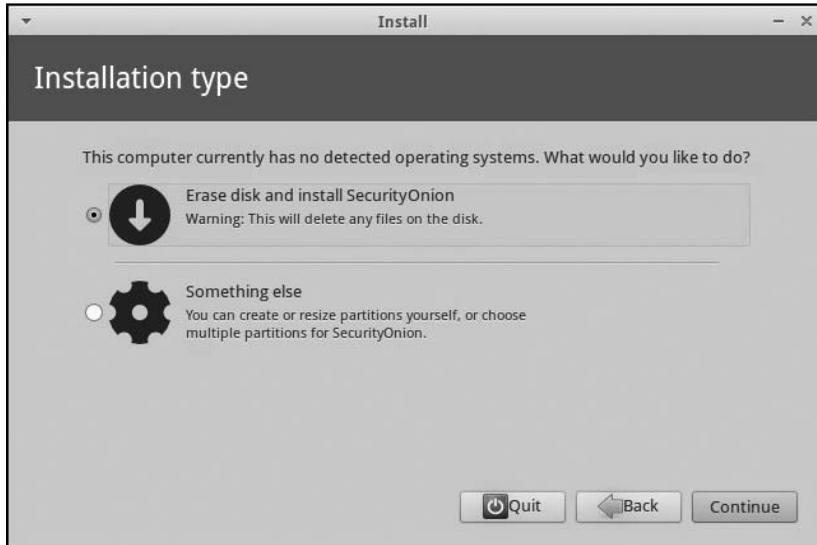
Figure 3-8: Choosing to erase the disk to install SO
