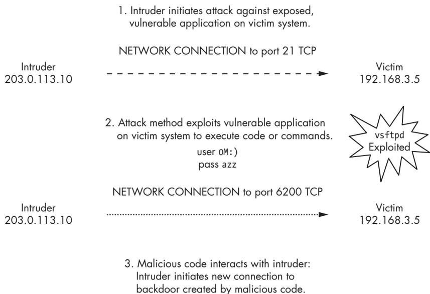
Figure 10-10: Server-side attack involving exploitation of vulnerable vsftpd server
