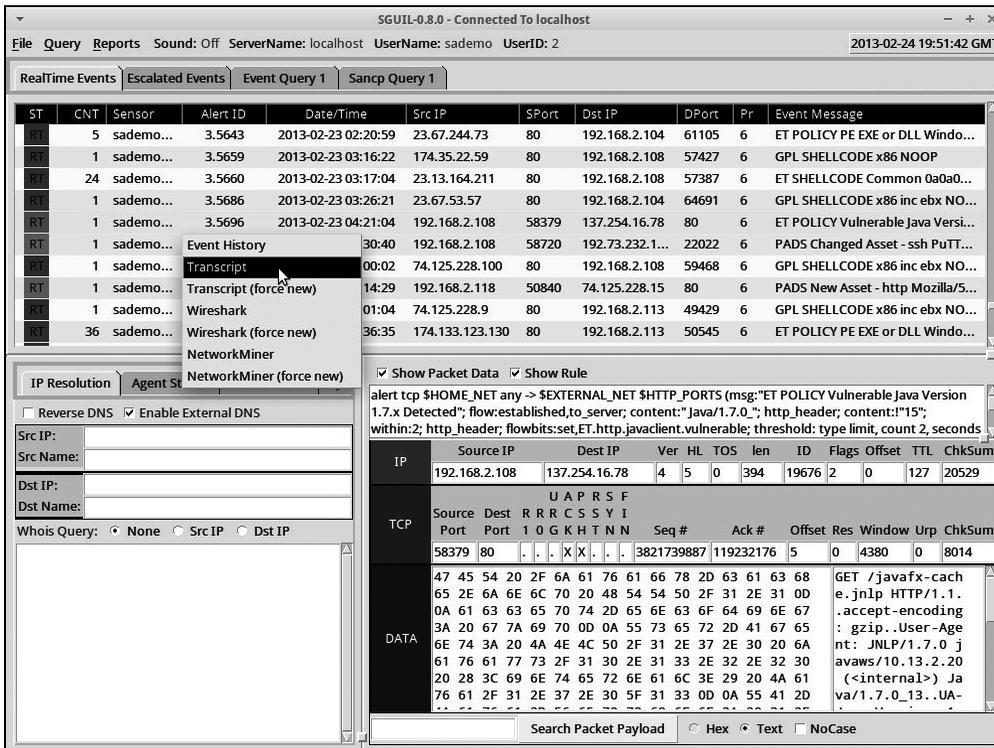
Figure 8-8: Pivoting from alert data to a transcript
