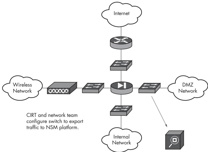
Figure 1-4: Simple network diagram and NSM platform
