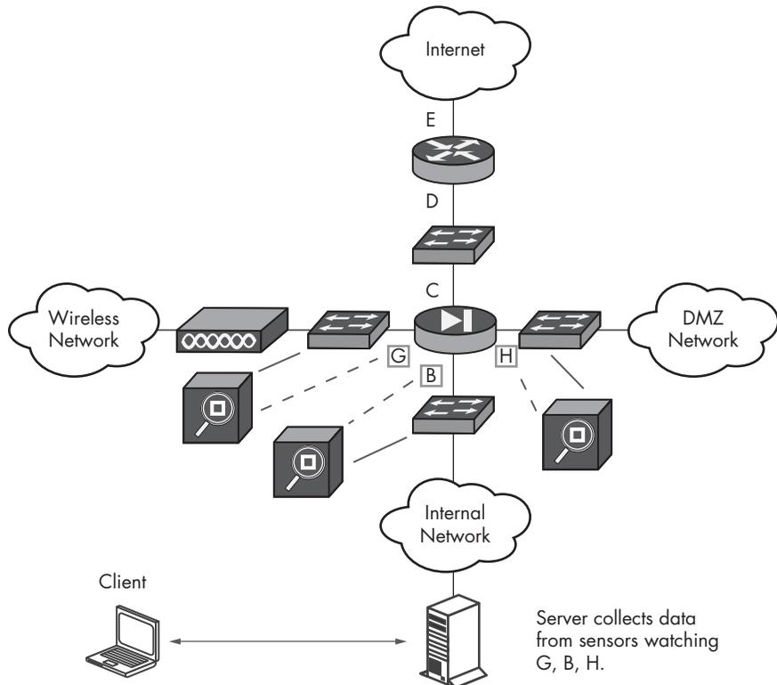
Figure 3-4: The SO server collects data from sensors watching network locations G, B, and H.
