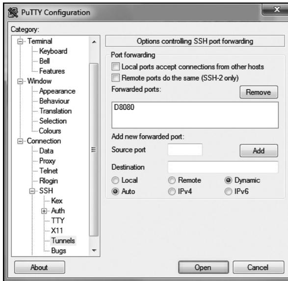
Figure 5-3: Configuring PuTTY for SSH port forwarding
