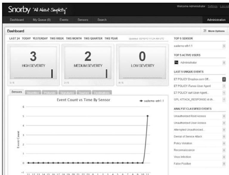
Figure 3-28: Snorby dashboard confirms stand-alone sensor operation.
